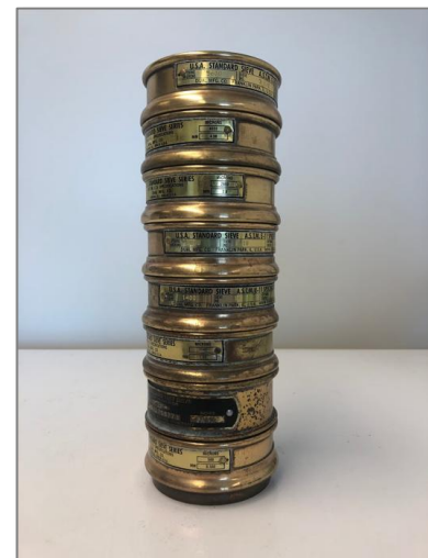
Figure 2. Nested tower of sieves. These sieves are made for measuring sediment size distribution and are available from scientific suppliers. See text.
