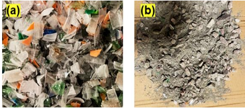
Fig.10 (a) PET waste following shredding, (b) Using PET in part to prepare a concrete sample. Adapted from Lukman Abubakar et al., 2024
