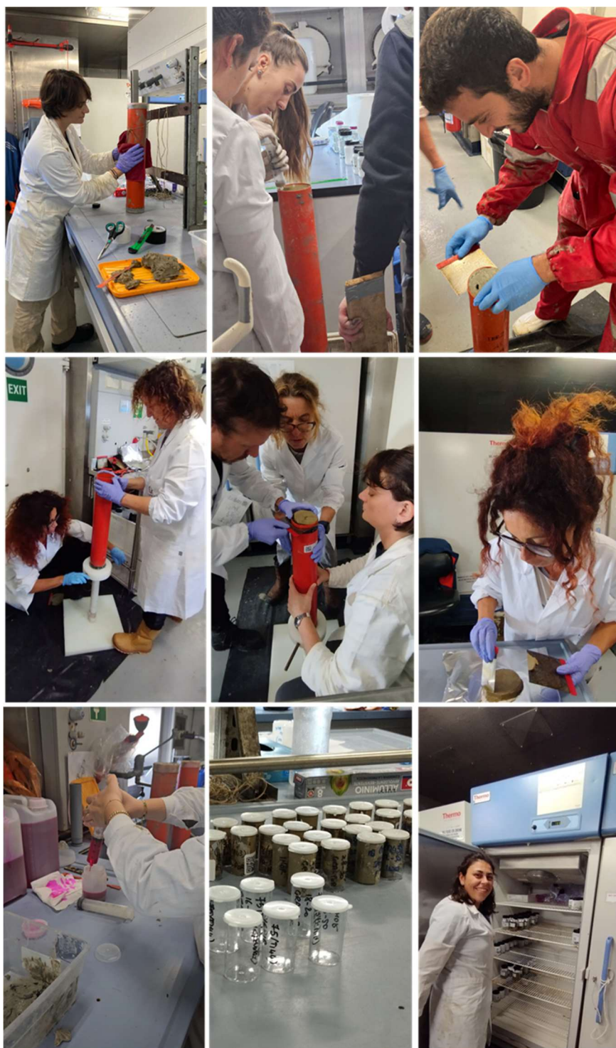
Figure 12. Wet Lab activities: core extrusion and slicing for physico-chemical analyses, Rose Bengal staining for foraminiferal analysis, aliquot subdivision, and storage.
