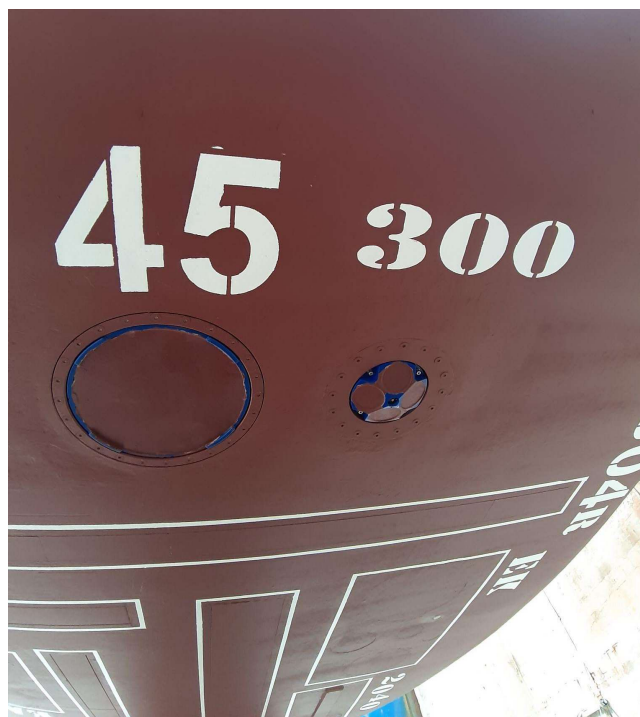
Figure 6. Locations of the two vessel-mounted ADCPs (Acoustic Doppler Current Profilers): the Teledyne RD Instruments (TRDI; Teledyne Marine Technologies Inc., Poway, CA, USA) Pinnacle (45 kHz) and Workhorse II Mariner (300 kHz), on the hull of the R/V “Gaia Blu”.
