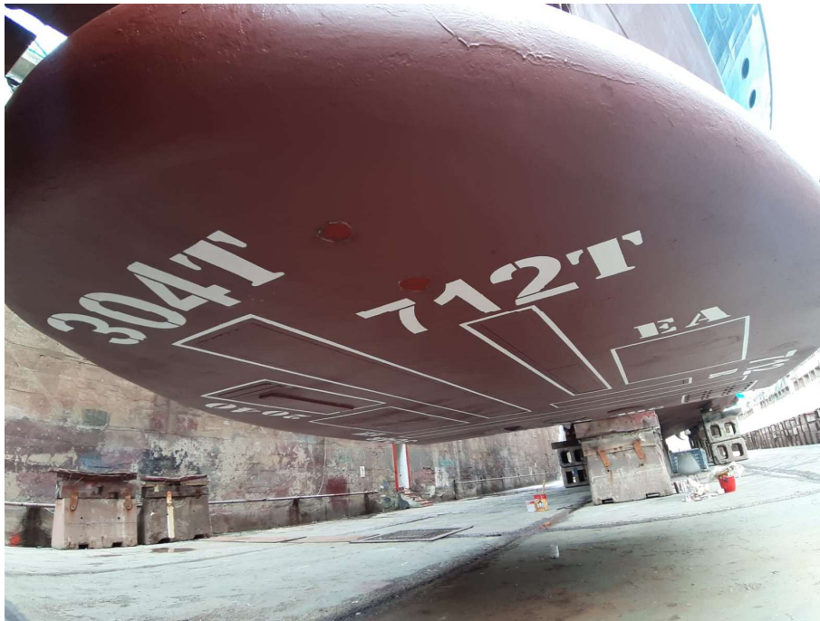
Figure 8. Location of the vessel-mounted Kongsberg Discovery (Kongsberg Gruppen ASA, Horten, Norway) EM 304 MKII and EM 712 MBESs (MultiBeam Echo Sounders), on the hull of the R/V “Gaia Blu”.
