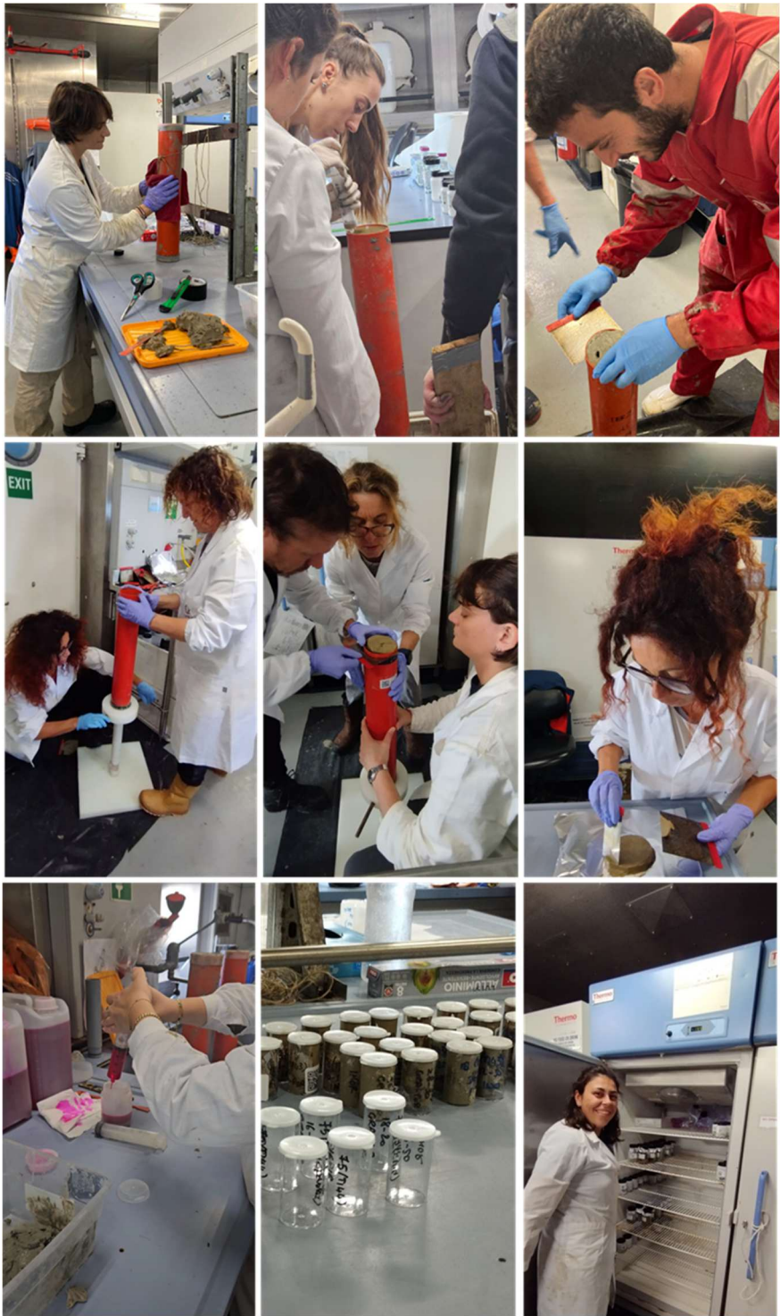
Figure 12. Wet Lab activities: core extrusion and slicing for physico-chemical analyses, Rose Bengal staining for foraminiferal analysis, aliquot subdivision, and storage.
