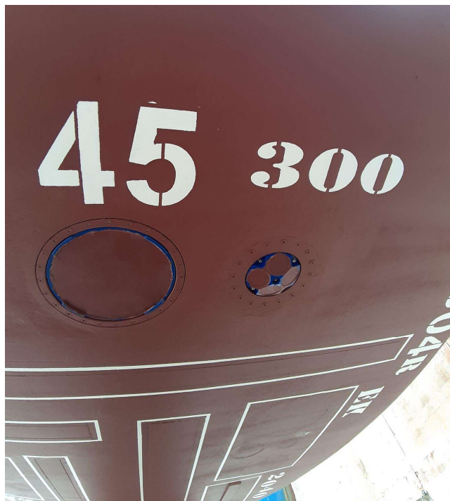
Figure 6. Locations of the two vessel-mounted ADCPs (Acoustic Doppler Currents Profilers): the Teledyne RD Instruments (TRDI; Teledyne Marine Technologies Inc., Poway, CA, USA) Pinnacle (45 kHz) and Workhorse II Mariner (300 kHz), on the hull of the R/V “Gaia Blu”.
