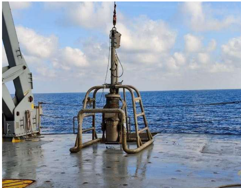
Figure 4. The box corer used on board for the sediment sampling.
