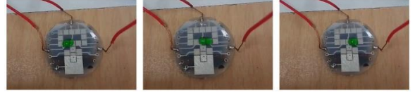
Figure 5: Motion of droplet on the EWOD system
