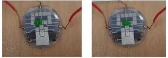
Figure 6: Distribution of a droplet on three electrodes.
