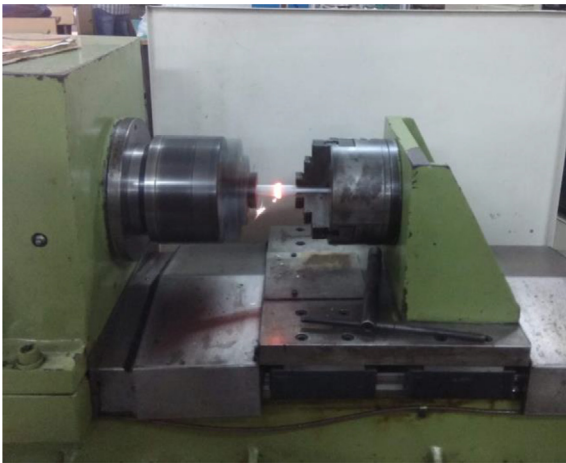
Fig 2. Fire point process of frictional welding.
