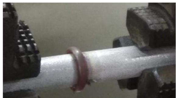
Fig 3. Friction Welded Samples.
