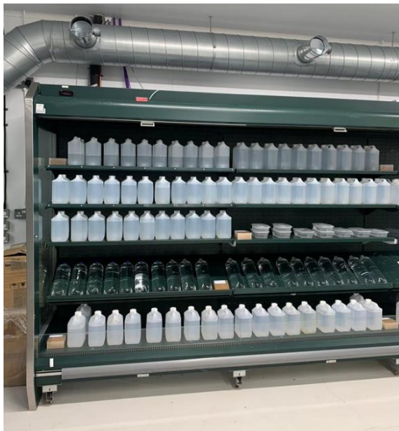
Figure 3: High temperature (HT) Monza display case used at Riseholme Refrigeration Research Centre.
