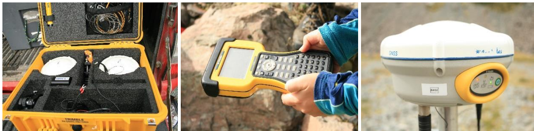
Figure 3.3.4.1. Shows the Trimble R6 GNSS system. (A) The Rover and Base station in its protective casing (B) The controller (C) Base Station
