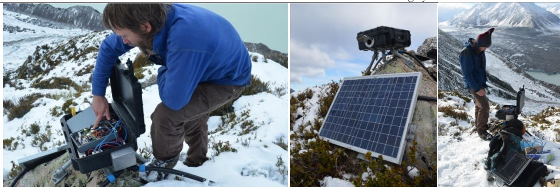
Figure 3.1.2. [LEFT] Shows the internal processor that communicates with the camera and specifies when to capture an image. [MIDDLE] The Tasman camera module is bolted into the bedrock as seen to mitigate camera movement. A 60W solar panel is used to power the entire setup. [RIGHT] Manual download of the images is time-consuming and only conducted when doing our 6 monthly maintenance check.
