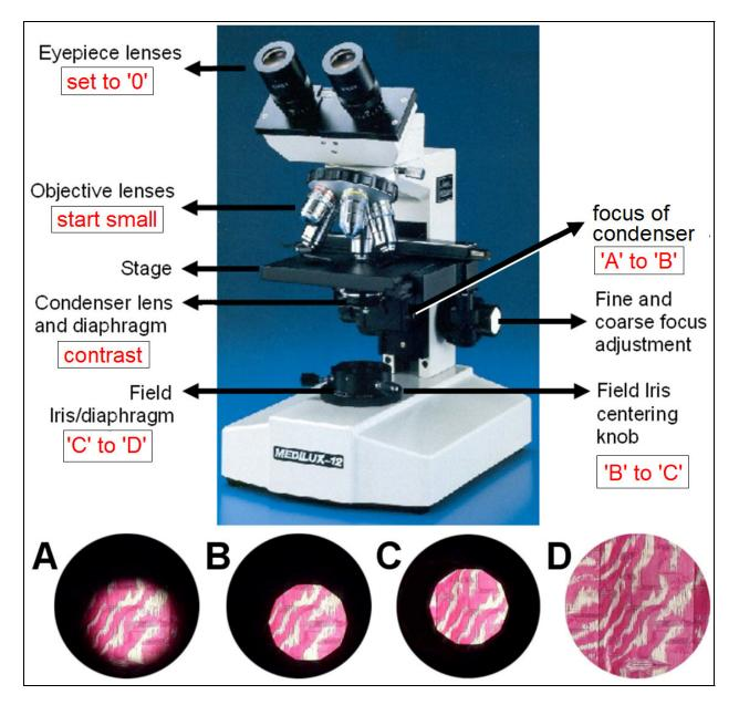
**Top:** A typical course microscope; arrows point at various parts that require proper setting (as indicated by boxed red text, respectively). **Bottom:** The step-wise procedure required to koehler the microscope: first close the field iris diaphragm, then perform step A-B with the condenser, B-C with the field iris centering knob, C-D with with the field iris diaphragm.
