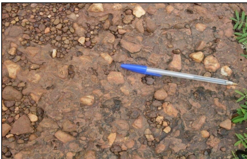
Fig. 4.11 Rounded and smooth quartz clasts in laterite: evidence of transportation - this is a clast-supported transported laterite located near pit SP002 with coordinate 518995E/1143689N.
