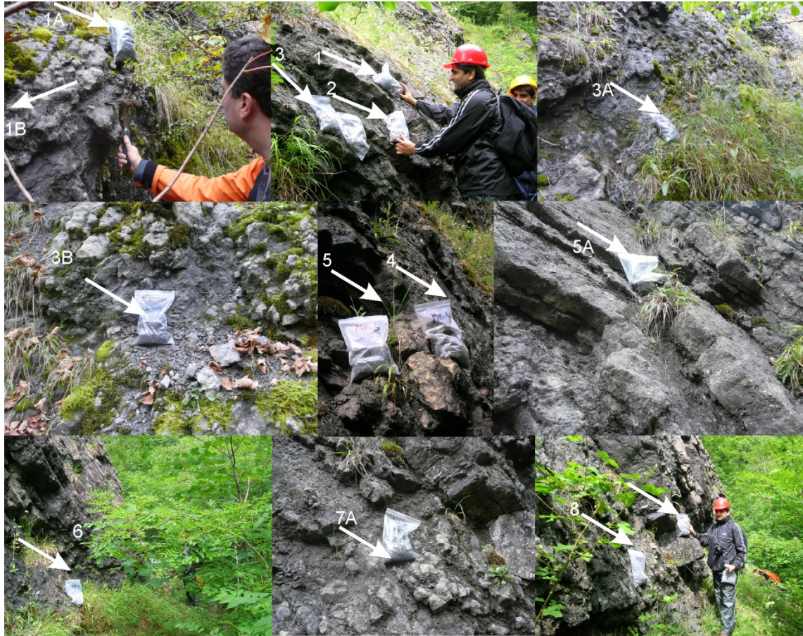
Figure 5. Craighead Quarry showing the inter-bedded limestone and shales (locality 6c) of the Craighead Limestone Formation. Sample horizons indicated by arrows.
