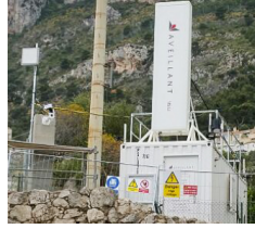
(a) Aveillant's Gamekeeper 16U counter-UAS radar [89].
