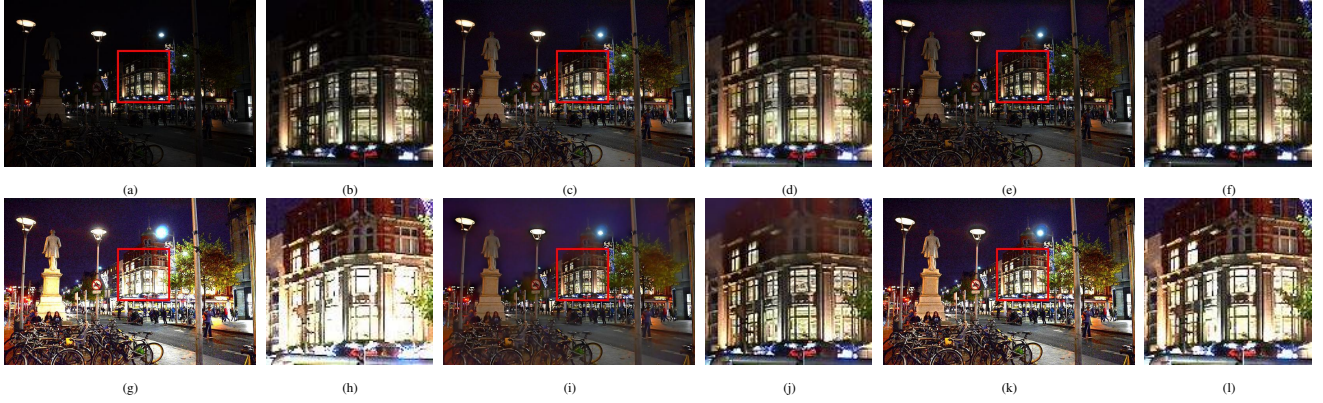
Fig. 3: Street. (a) Input image; (b) Marked patch of (a); (c) Result of PIRE; (d) marked patch of (c); (e) Result of WRIE; (f) Marked patch of (e); (g) Result of LIME; (h) Marked patch of (g); (i) Result of SRLIME; (j) Marked patch of (i); (k) Result of proposed method; (l) Marked patch of (k).
