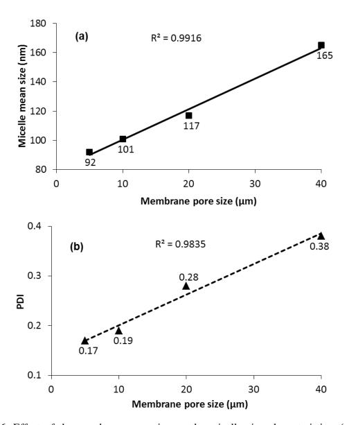
**Figure 6.** Effect of the membrane pore size on the micelle size characteristics: (a) mean micelle size, and (b) PDI of the micelles. The membrane pore spacing is  $200 \, \mu m$  and other conditions are specified in Table 4.
