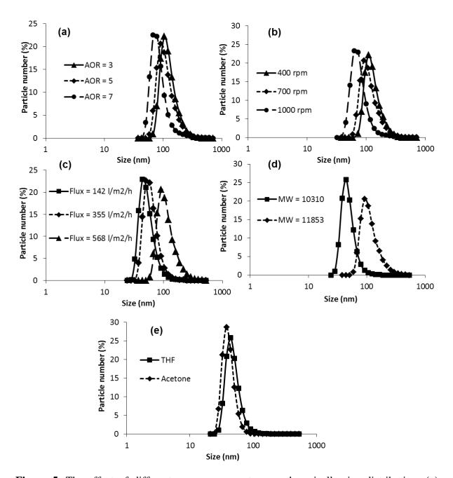
**Figure 5.** The effect of different process parameters on the micelle size distribution: (a) Aqueous to organic phase volume ratio, AOR, (b) Agitation speed, (c) Transmembrane flux, (d) Polymer molecular weight, and (e) Type of the organic solvent. Other conditions are specified in Table 3.
