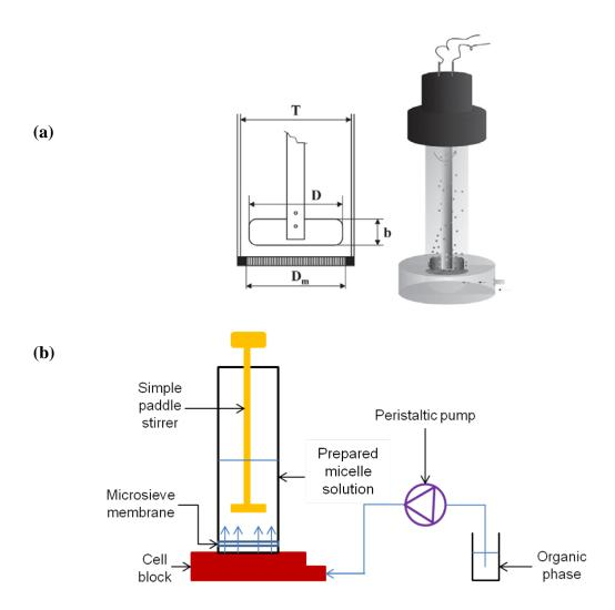
**Figure 1.** (a) Schematic illustration of the stirred cell with simple paddle stirrer above a flat disc membrane (b = 12 mm, D = 32 mm,  $D_m = 33$  mm, and T = 40 mm). (b) Schematic diagram of the experimental set-up.
