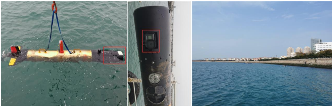
10 Fig. 5 The experimental scene in Jiaozhou Bay, Qingdao. Three GoPro 8 Hero Black cameras are mounted on the 11 head of AUV. Tow areas marked by red rectangles are the head of AUV and the GoPro 8 Hero Black camera we 12 used in the experiments, respectively. 13
