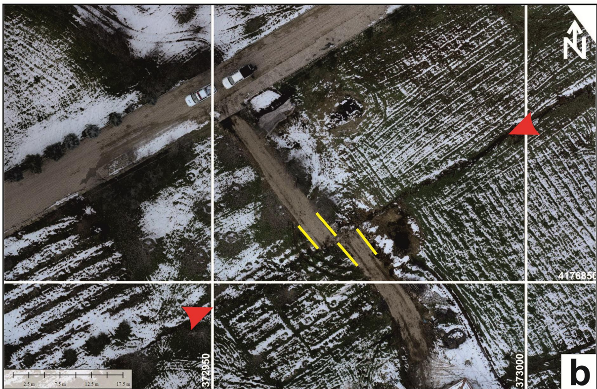
Figure S9. Left-lateral displacements on a road (location 51, Table1 in the main text; high-resolution map produced with RTK-drone).
