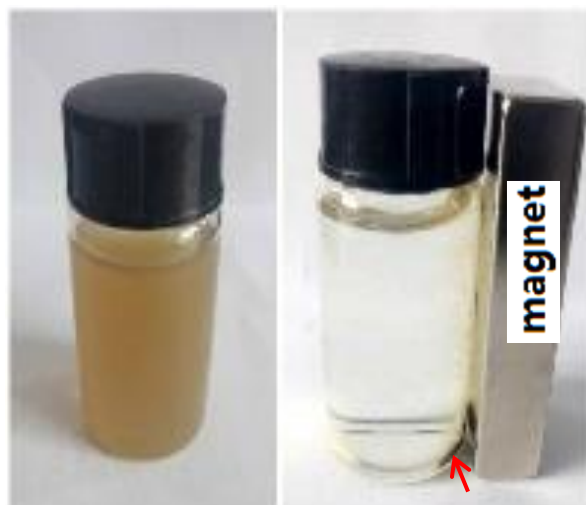
Fig. s1. Image of the MDSHSs separated from the solution by a magnet.
