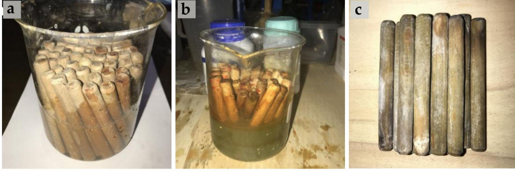
Figure S2. Pretreatment methods and the process of the wood dowel, (a) Dowels impregnated with an oxidising agent; (b) impregnation of dowels with sulphonating agents; (c) Spraying with an ethanolic solution of zinc acetate.
