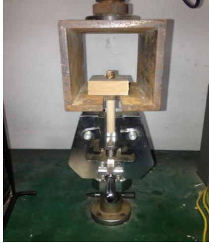
Figure S3. Diagram of bonding strength test.
