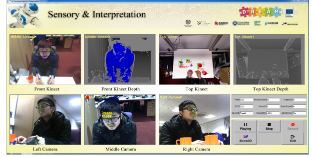
Fig. 5. The Graphical User Interface (GUI) component used by the therapist to control the sensory system. On the right bottom side, the control button panel can be used to control the preview and record function. The “Show3D” button is used to present all sensitised data in a unified 3D world coordinate.
