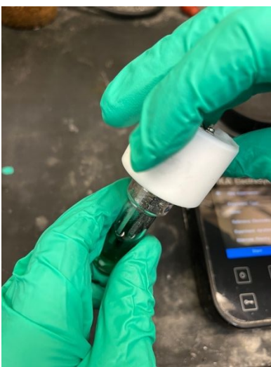
Left: Attachment of the cap to the Electrasyn 2.0 vial. Center: Attached vial to the Electrasyn 2.0. Right: Start of the reaction. Permitted use of logo is credited to IKA.
