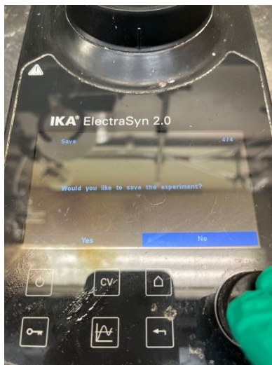
Left: Select “No” when prompted about alternating polarity. Center: Select “No” when asked to save experiment. Right: Addition of silver nitrate to the homogenous reaction solution. Permitted use of logo is credited to IKA.
