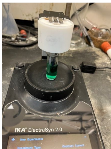
Left: Attachment of the cap to the Electrasyn 2.0 vial. Center: Attached vial to the Electrasyn 2.0. Right: Start of the reaction. Permitted use of logo is credited to IKA.
