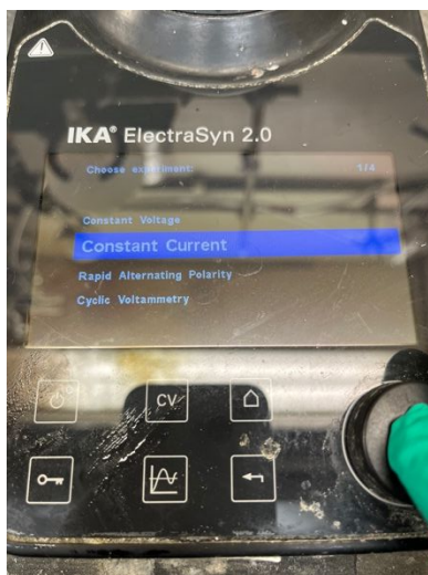
Left: Select “New Experiments”. Center: Select “Constant Current”. Right: Set the current to 12 mA. Permitted use of logo is credited to IKA.
