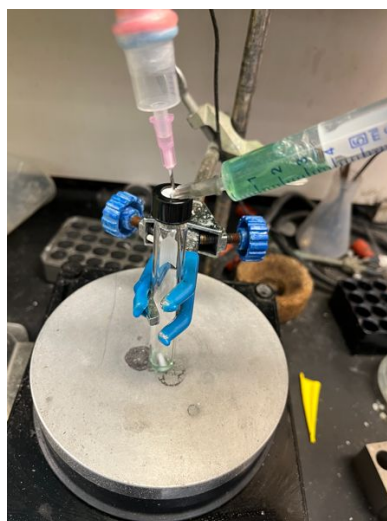
Left: Silver nitrate weighed out in a 5 mL Electrasyn vial. Center: Vacuum and purging of the Electrasyn vial with argon. Right: Transfer of of the catalyst solution via syringe to the in situ RAE synthesis.
