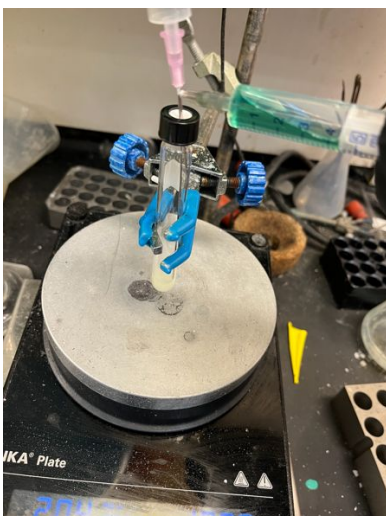
Left: Addition of the catalyst solution to the in situ RAE synthesis. Center: Combined catalyst and RAE solutions. Right: Combined solution added to the Electrasyn vial with silver before electrolysis. Permitted use of logo is credited to IKA.
