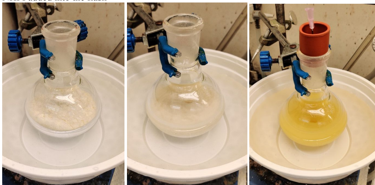
Left: Flask submerged into a water bath Center: THF is added (125 mL). Right: Reaction Mixture after DIC addition.
