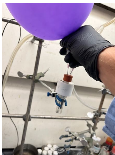
Left: Silver nitrate weighed out in a 5 mL Electrasyn vial. Center: Vacuum and purging of the Electrasyn vial with argon. Right: Transfer of of the catalyst solution via syringe to the in situ RAE synthesis.
