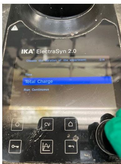
Left: Select “No” when prompted about a reference electrode. Center: Select “Total Charge”. Right: Set the scale to 0.4 mmol and the “equivalents of electrons” to 2.5 F/mol. Permitted use of logo is credited to IKA.
