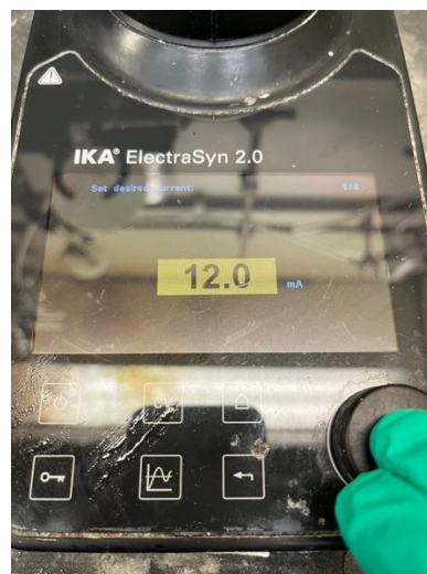
Left: Select “New Experiments”. Center: Select “Constant Current”. Right: Set the current to 12 mA. Permitted use of logo is credited to IKA.
