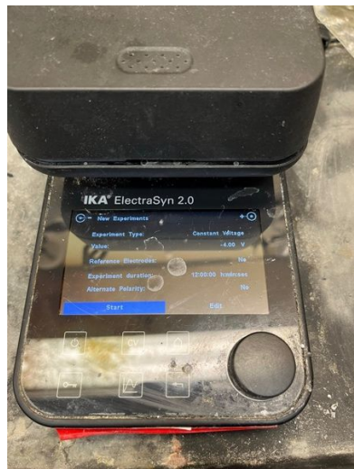
Left: E-hive prior to the start of the electrolysis. Center: Closed E-hive. Right: Electrochemical parameters for the E-hive (-4.0V applied potential for 12 h). Permitted use of logo is credit to IKA.
