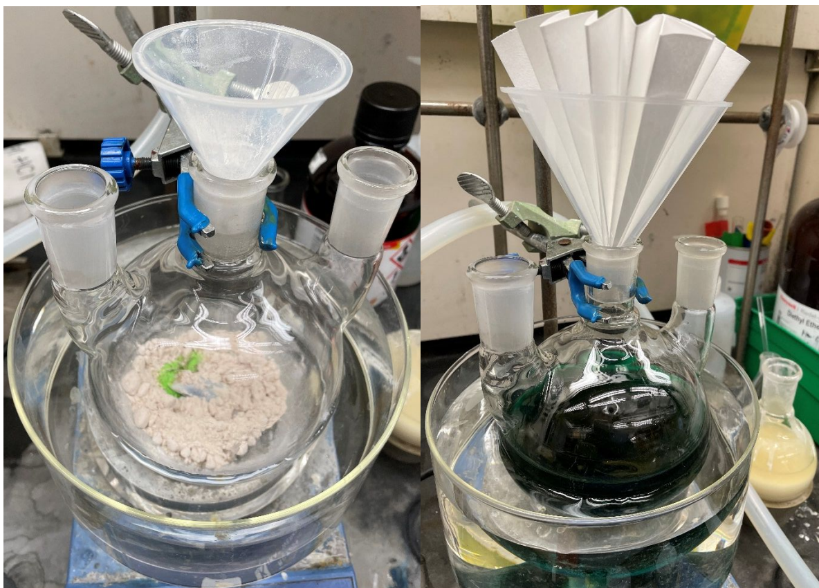
Left: 1L, Three-necked round bottom flask charged with aryl iodide, \text{NiCl}_2 \cdot 6\text{H}_2\text{O} , 2,2'-bipyridine and \text{LiCl} , submerged in a water bath. Right: After addition of NMP (625 mL).
