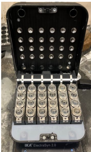
Left: E-hive prior to the start of the electrolysis. Center: Closed E-hive. Right: Electrochemical parameters for the E-hive (-4.0V applied potential for 12 h). Permitted use of logo is credit to IKA.
