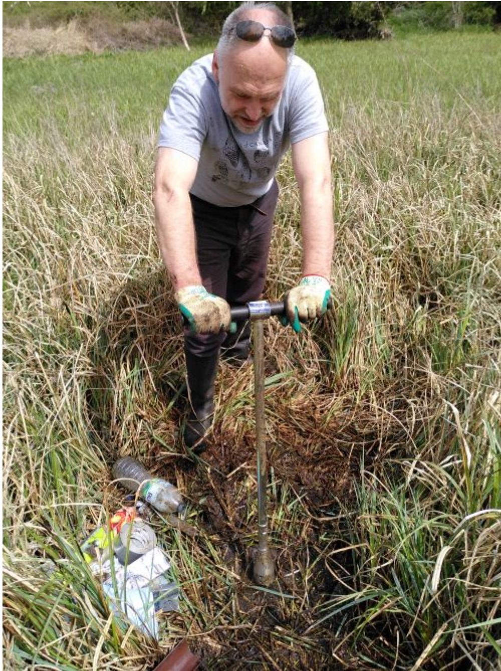
Figure 3: Taking peat/sediment samples using a Russian corer at Daisy Banks Fen, Oxfordshire
