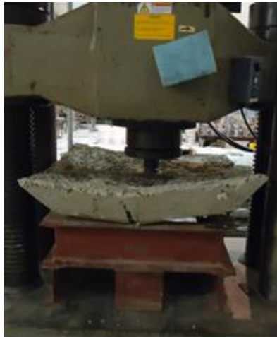
621 622 Figure 2: Square panel test according to EN 14488-5.
