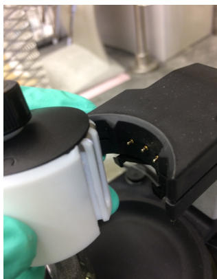
(Left) The electrochemical cell was plugged into ElectroSyn 2.0. (Middle) Select New experiments. (Right) Select Constant Current.
