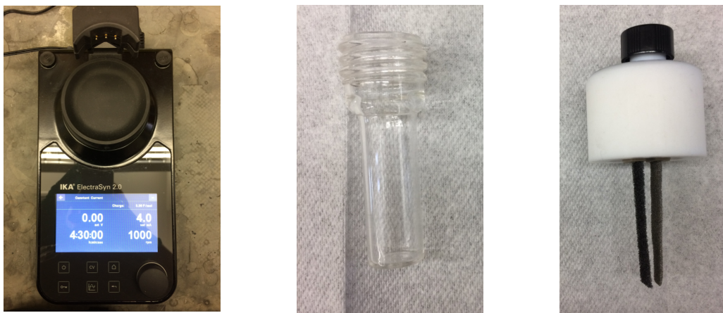
(Left) ElectraSyn 2.0. (Middle) ElectraSyn 2.0 vial (5 mL). (Right) ElectraSyn 2.0 cap equipped with RVC (left side) and Nickel electrodes (right side).
