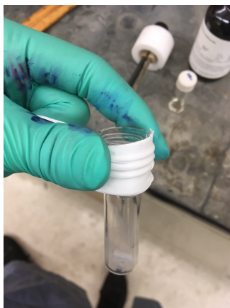
(Left) Materials used in the reaction. (Middle) Wrapping Teflon tape helps to keep a good sealing during a reaction. (Right) The appearance of the mixture after the addition of all solid components.
