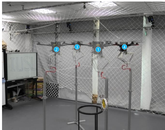
Fig. 1: Aerial weaving by an aerial manipulator. The experimental video is available at https://youtu.be/QMjGtBCUi-E .
