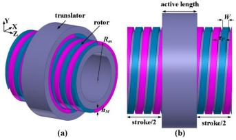
Fig. 1. Views of an idealized TROMAG; (a) 3D view; (b) side view.
