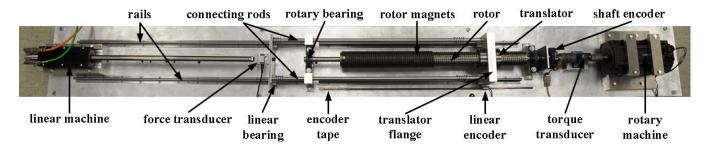
Fig. 3. Experimental TROMAG set-up assembly
