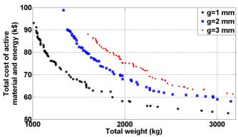
Fig. 14. Pareto-optimal fronts of 100 kW LTMs with different values of air gap length
