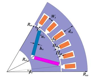
Fig. 5. One pole of the V-shaped rotary IPM and its geometrical design variables
