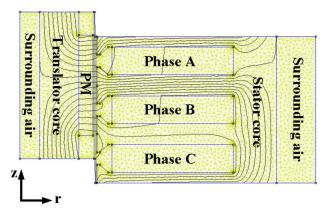
Fig. 11. Mesh and flux lines of LTM design #2 in magnetic FEA
