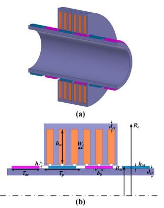
Fig. 6. A PM LTM and its geometrical design variables; (a) cut-away view, and (b) 2D view
