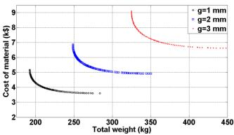
Fig. 15. Pareto-optimal fronts of TROMAGs with different values of air gap length
