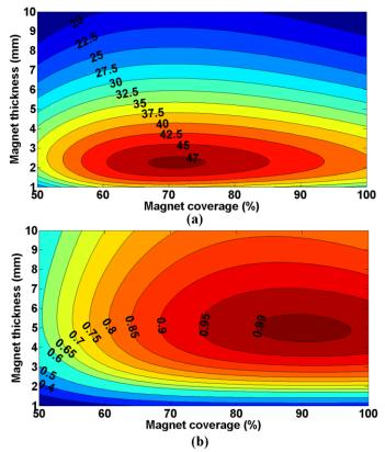
Fig. 7. Contour plots of variations of force per cost and force per weight of a TROMAG with zero stroke vs magnet thickness and coverage; (a) force per cost (N/\$), (b) force per weight (kN/kg).
