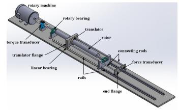
Fig. 2. Schematic of a TROMAG set-up assembly.
