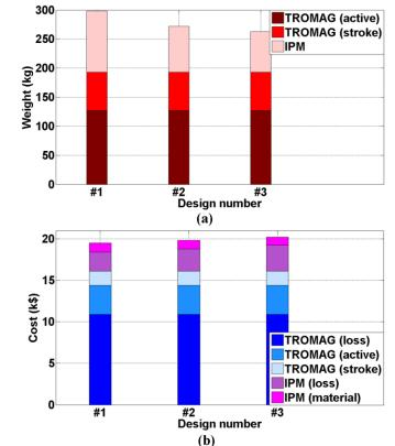
Fig. 10. Weights and costs of three designs of a 100 kW MITROMAG; (a) weight, and (b) cost of material and energy
