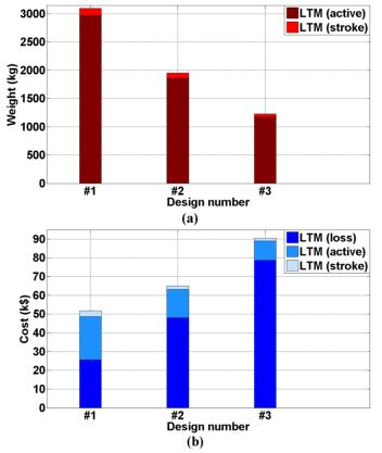
Fig. 12. Weights and costs of three designs of a 100 kW LTM; (a) weight, and (b) cost of material and energy.
