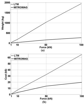
Fig. 13. Comparison of MITROMAG and PM LTM at four levels of force with similar speed and stroke; (a) weight, and (b) cost
