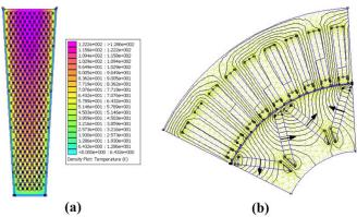
Fig. 9. Thermal and magnetic FEA of IPM design #2; (a) a populated slot and its temperature distribution, (b) mesh and flux lines in magnetic FEA.
