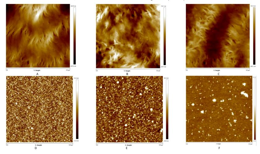
SM2: PFQNM images, representing the indentation modulus image and the corresponding cross section analysis for A) PHBHV sample, B) PDMS sample and C) PDMS/PDMS-PEG sample
