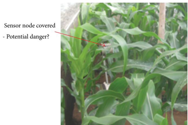
FIGURE 13: Sensor node being covered by maize plants.
