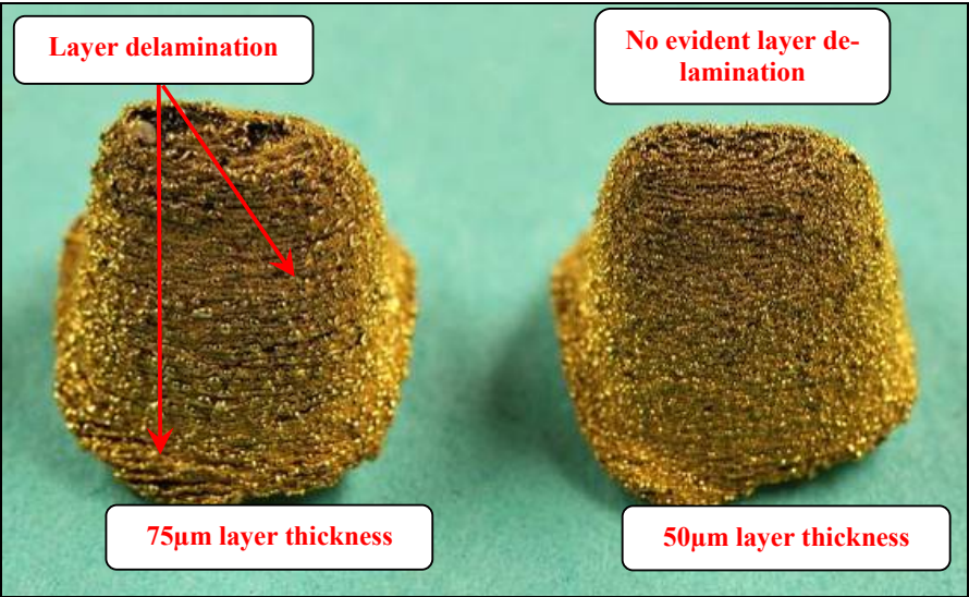
Figure 9-21: Gold premolar dental parts produced with 75 \mu\text{m} and 50 \mu\text{m} layer thickness
