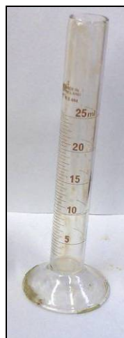
Figure 6-9: Standard 25\text{cm}^3 graduated glass cylinder
