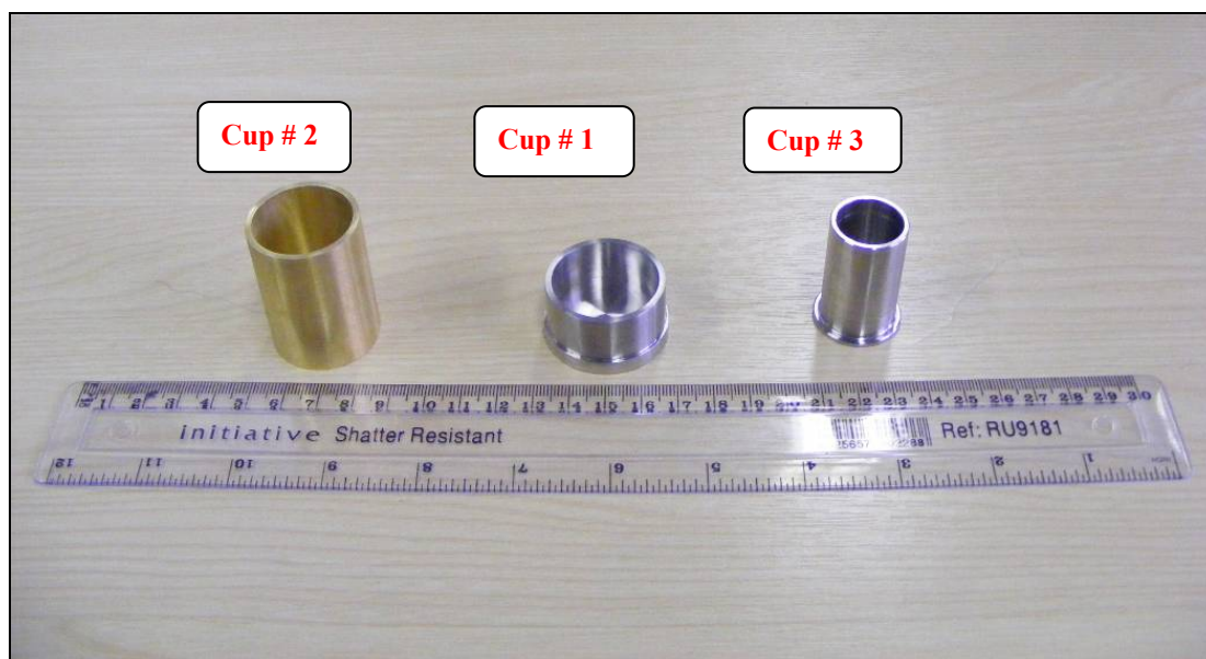
Figure 6-7: Apparent density cups with different aspect ratios
