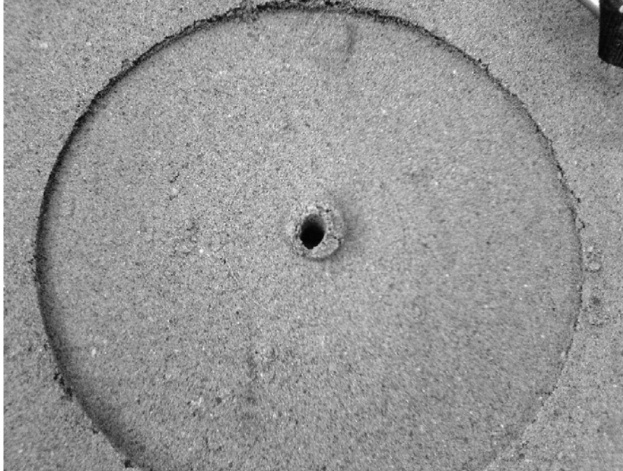
FIGURE 5. The Effect of Repeated LWD Impacts on the Sand Layer, Showing Permanent Deformation Under the Plate and Disturbance Under the Geophone Foot.
