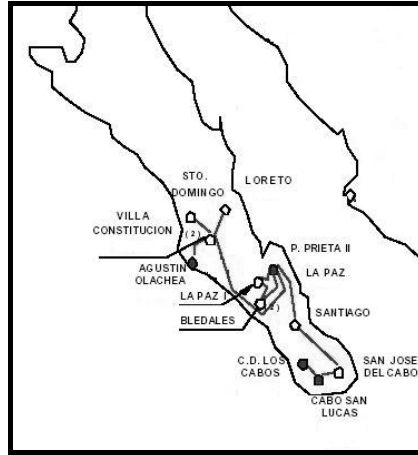
Figure 2. BCS's electricity transmission grid. Source:[9]
