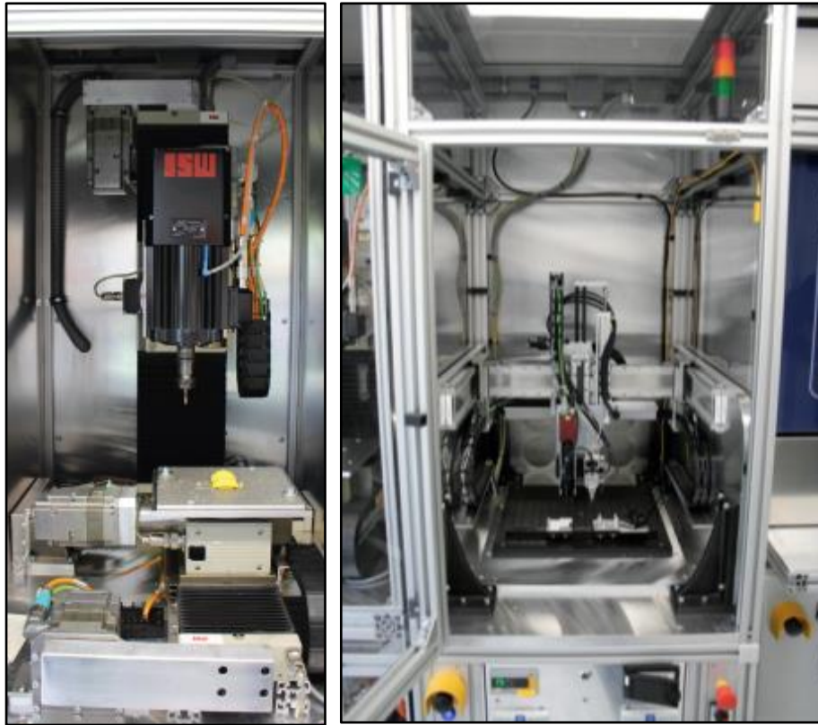
Figure 13: CNC-Milling module (left) and Assembly module (right)
