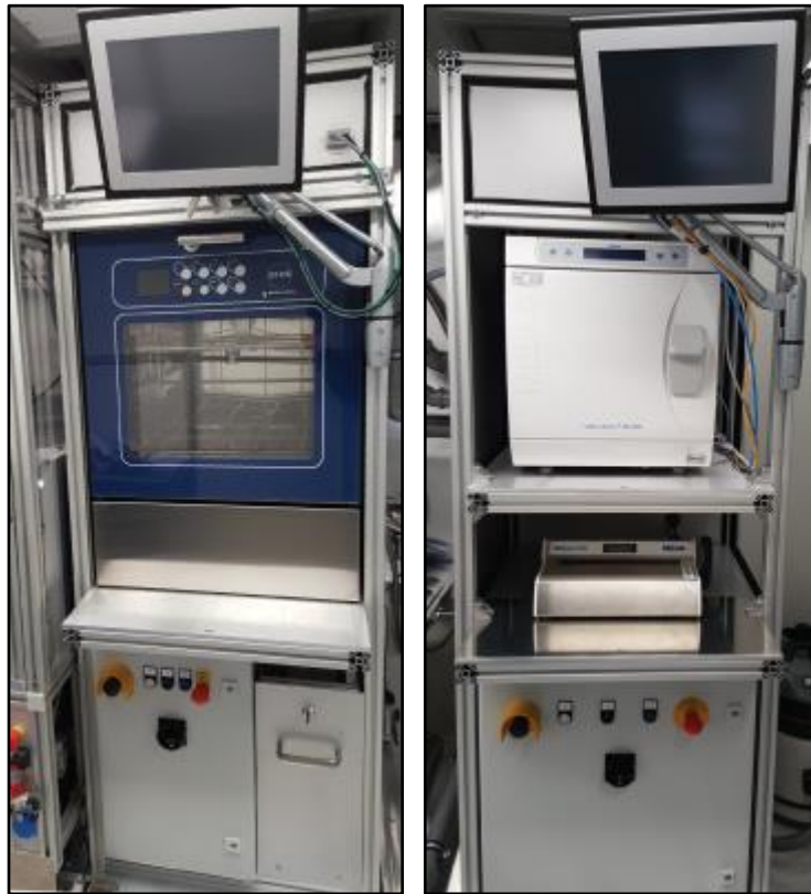
Figure 14: Cleaning module (left) and sterilization module (right)
