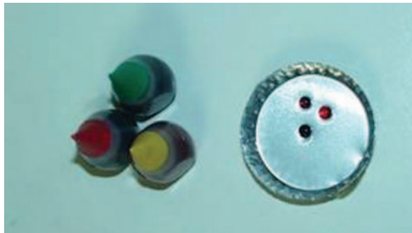
FIGURE 6. Three drops of food dye, red, green, and yellow floating in HFE-7200.
