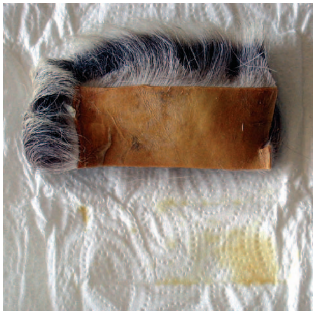
FIGURE 20. Residues left on the paper tissue after extraction of the caribou fur with SC-CO 2 .
