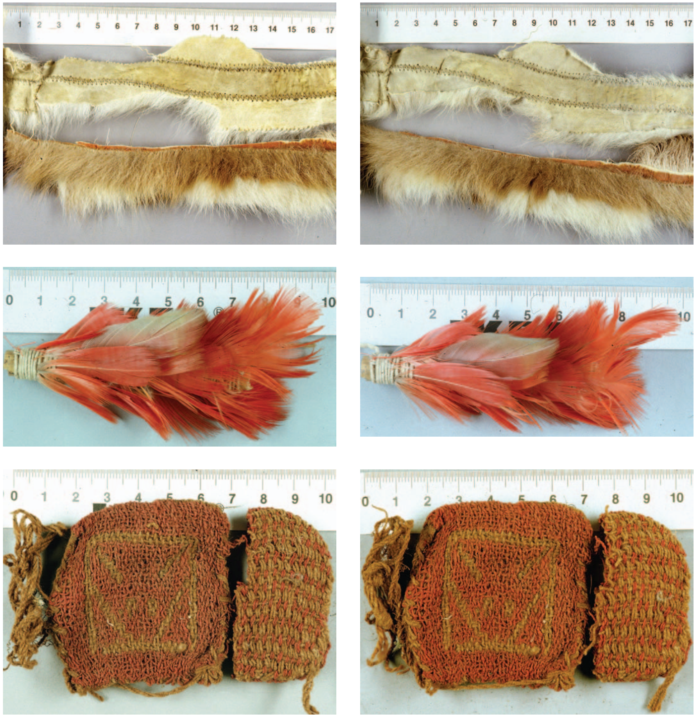
FIGURE 17. Left column, from top to bottom, samples of fur, bundle of feathers, and wool tissue before extraction. Right column, samples after extraction with SC-CO 2 .
