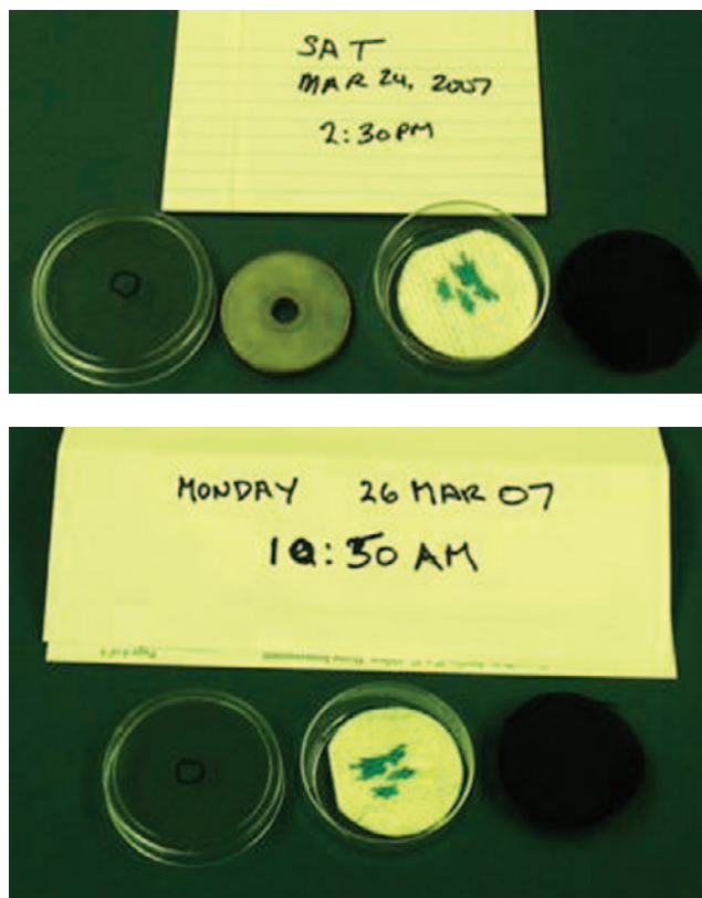
FIGURE 4. In the absence of a diffusion medium, no transfer is observed between the contaminated fabric and the activated carbon coupon. Top, at the beginning of the test; bottom, after 44 hours of contact between the contaminated fabric and the activated carbon coupon but without HFE.
