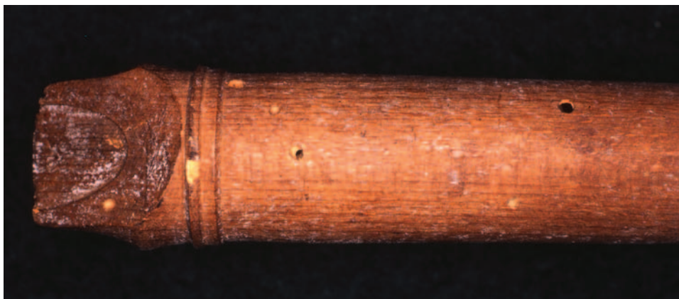
FIGURE 2. Dichlorodiphenyltrichloroethane (DDT) spot deposits on a flute from the Museum of Musical Instruments in Leipzig, Germany.
