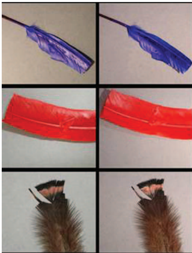
FIGURE 1. Effect of supercritical carbon dioxide (SC-CO 2 ) extraction on color and texture of three feathers: left, before extraction; right, after extraction.
