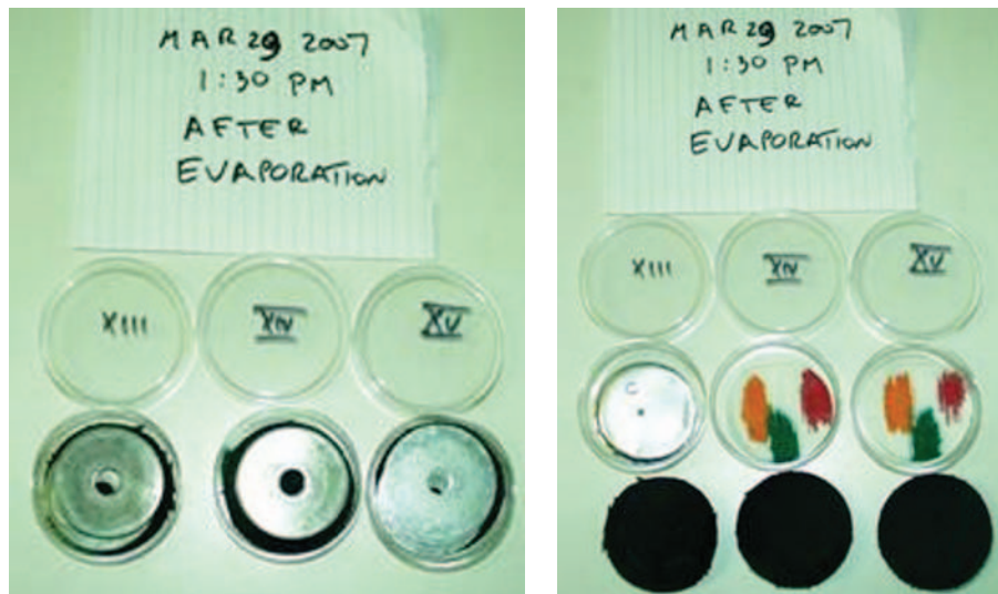
FIGURE 11. Left, petri dishes of Figure 10 after evaporation of the solvent before dismantling the stacks. Right, view after removal of metal washers and the activated carbon fabric layer.
