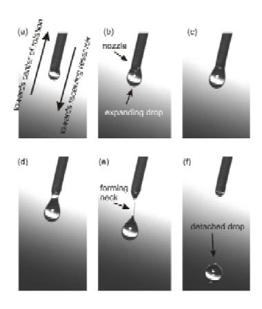
Figure 8. Sequential stroboscopic images of the droplet formation process at 25 Hz: (a)-(c) a liquid (2% chitosan solution) is subjected to a centrifugal pseudo-force field that leads to a droplet growth at the end of the nozzle. (d)-(e) The surface tension of the liquid favours a spherical shape which leads to a thinning neck between the droplet and the remaining liquid in the nozzle. (f) Finally, the droplet detaches and moves towards the receiving reservoir.
