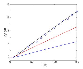
FIG. 6. The increase of the resistivity,  $\Delta \rho(T)$ , with temperature at B=0 measured on a 15  $\mu m$  Hall bar with a single gate (open blue circles) and the corresponding calculation (solid black curve) for  $n_s=3.2\times 10^{12}$  cm<sup>-2</sup>. The blue and red curves show separately the calculated contribution of the LA and TA phonons respectively to the resistivity,  $\rho^{\rm LA}(T)$  and  $\rho^{\rm TA}(T)$ .
