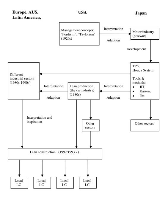
Figure 1: Schematic overview of the diffusion of lean production. – Schematic overview, only main ways (arrows) shown.
