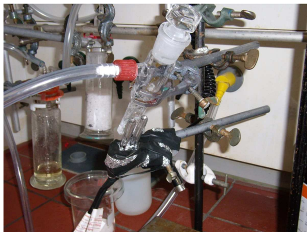
Figure S1. The quartz reactor and the UV lamp used for the photochemical grafting of 5-Hexen-1-ol on ITO substrate.
