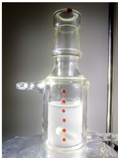
Figure S1 – Custom-made jacketed cell for sample preparation. Red dots inside the jacket serve as graduation marks. The circulating water bath connects by hose barbs.
