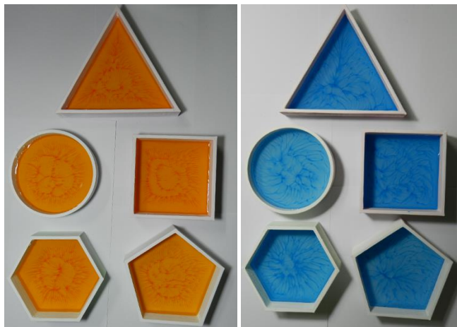
Figure 7S Left: Patterns formed by indigo carmine at a cross-sectional area of 50 \text{ cm}^2 and a depth of 1 cm. Right: Patterns formed by methylene blue at a cross-sectional area of 50 \text{ cm}^2 and a depth of 1 cm.
