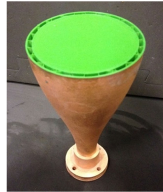
Fig. 1. Photograph of additively manufactured profiled horn with dielectric loading after electroplating.
