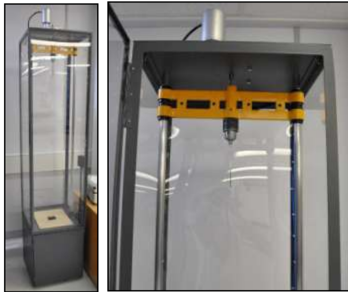
Figure 2 : In-house manufactured impact rig to HOSDB requirements.
