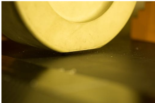
Figure 2. 4mm Clearance between wheel and floor in the LUMS wind tunnel.
