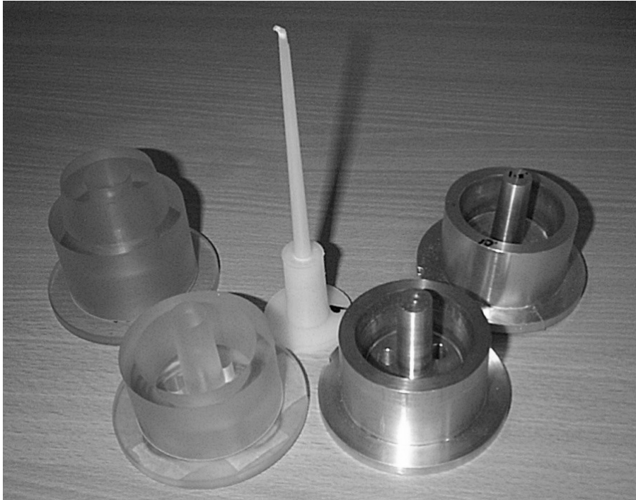
Figure 2. Cores and cavities used along with a complete moulding.
